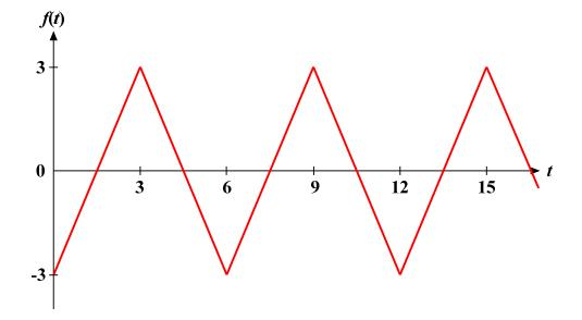
The red waveform shown below is periodic. Determine its average and effective (rms) values.
